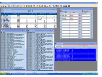
ENVIDAS software is a flexible, easy-to-use, turnkey application software that turns a PC with a data acquisition card into an intelligent environmental data acquisition system. It has the following features:
